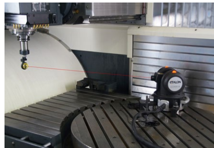
Complete measurement of rotary table axis of a machine tool
