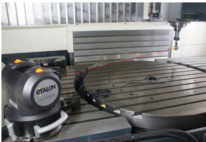
Complete measurement of linear machine tool axes
