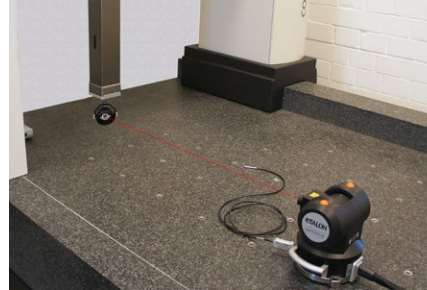
Testing and verification of a CMM according to ISO 10360-2
